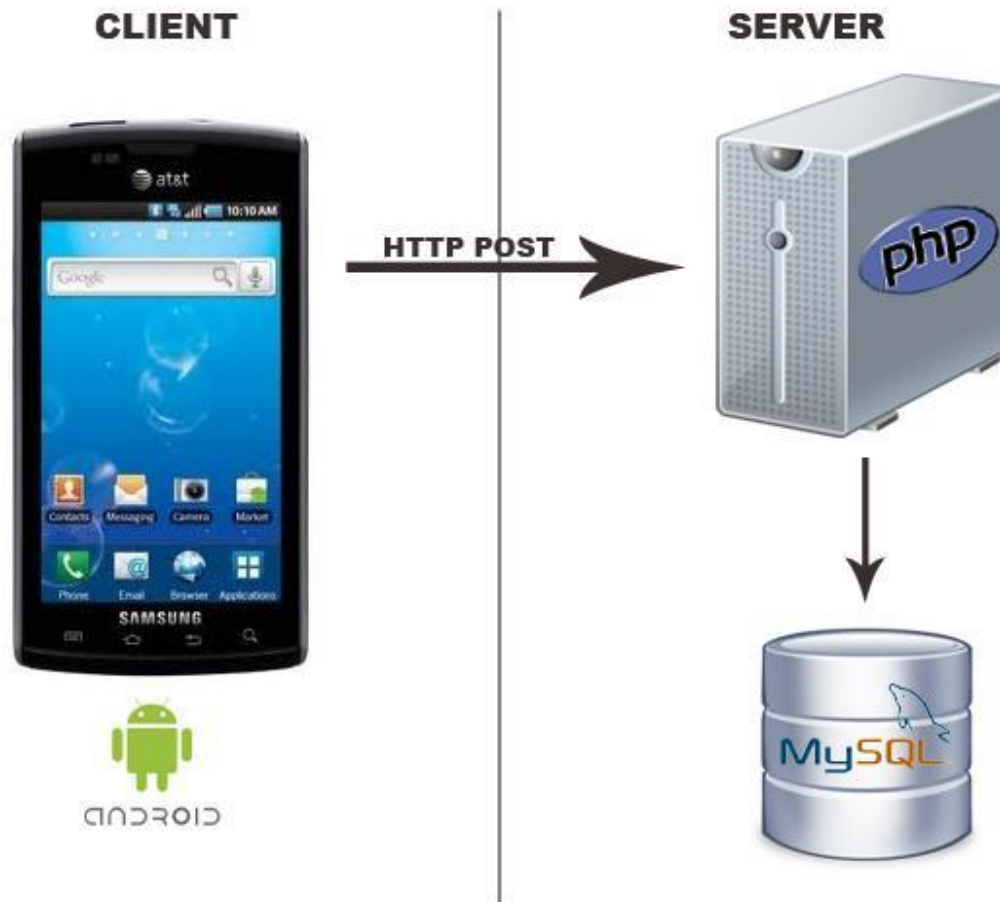
Figure 11 - A model diagram describing the system architecture in the client and server side ends
