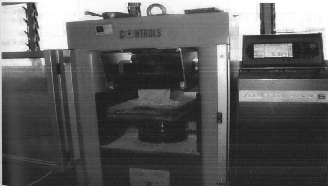
Figure 20: Compressive Strength Testing at Ambient Temperature
