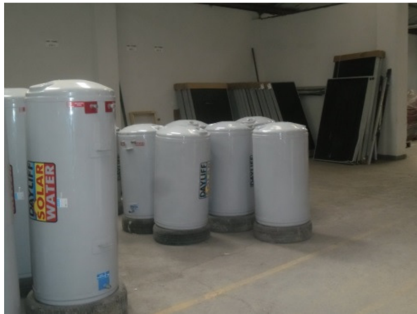
Figure 1.3: Galvanized Insulated Tank and Solar Collector ( Courtesy: D&S, 2014)
