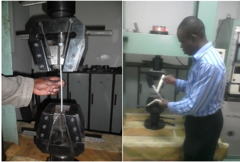
Figure 3.12: Tensile test with difference moisture content.
