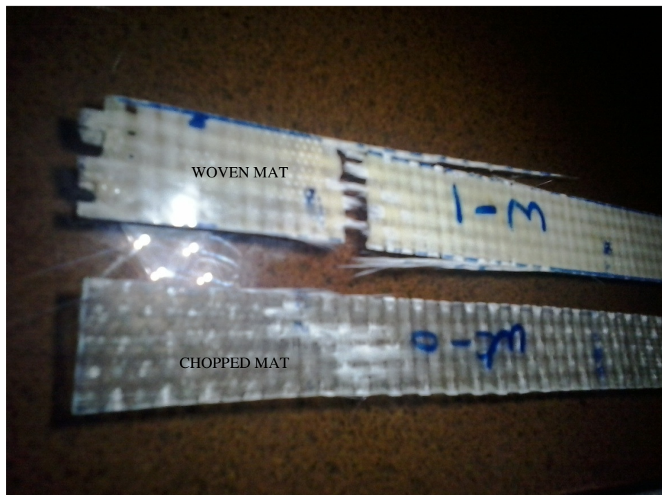
Figure 4.2: The specimens after tensile tests failure modes
