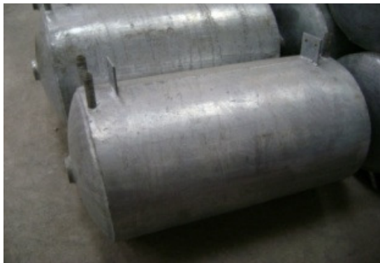
Figure:1.1:Galvanized Uninsulated Tank ( Courtesy: D&S, 2014)
