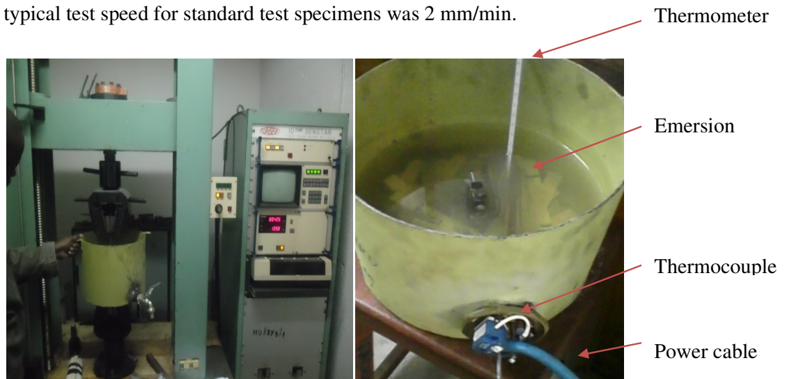
Figure 3.13: Hygrothermal Tensile Tests in the UoN Mechanical lab.
