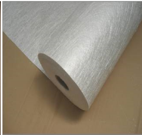
Figure 2.5: E-Glass chopped strands mat 450 GSM, (Courtesy: D&S 2012)
