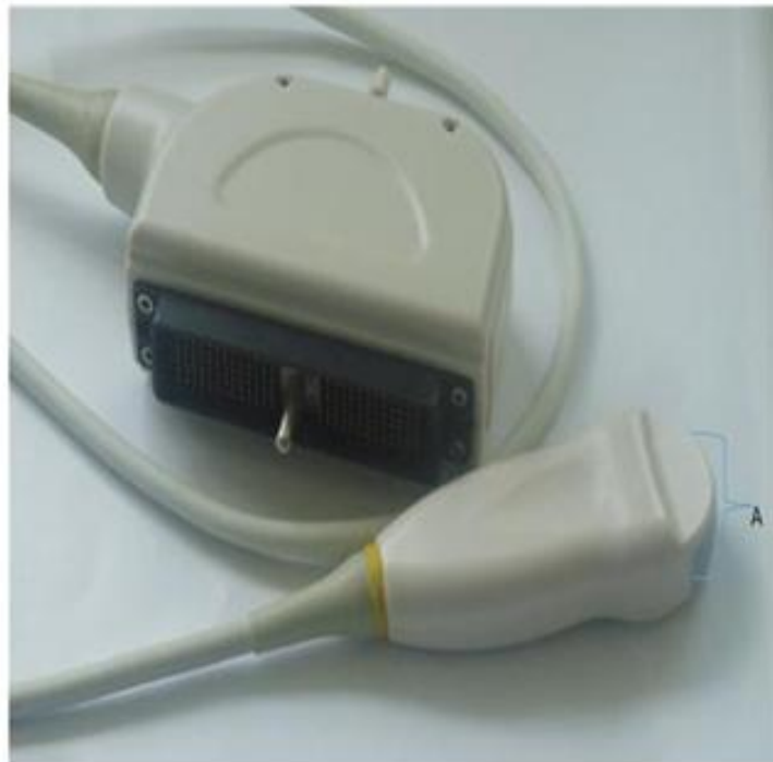
Figure 3. 1: Photograph of a convex array probe of the machine used in the study. A-footprint.
