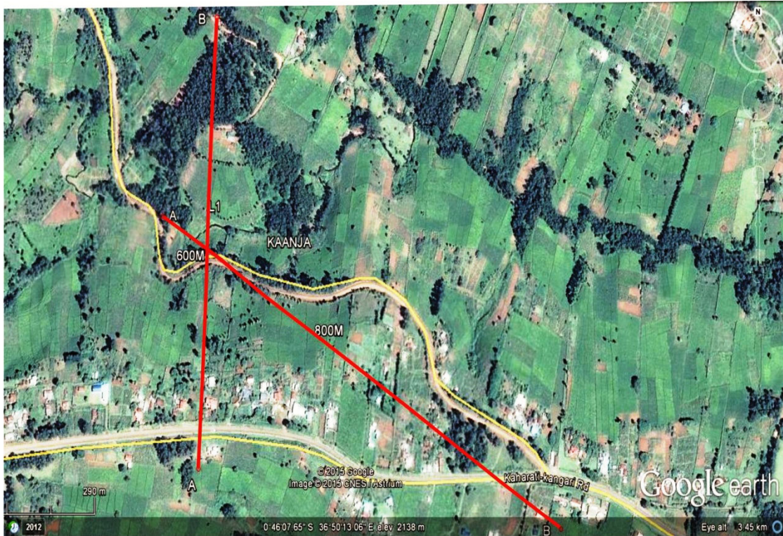
Figure 5.22. Google earth map of Kaanja site, showing the two ERT profile layout
