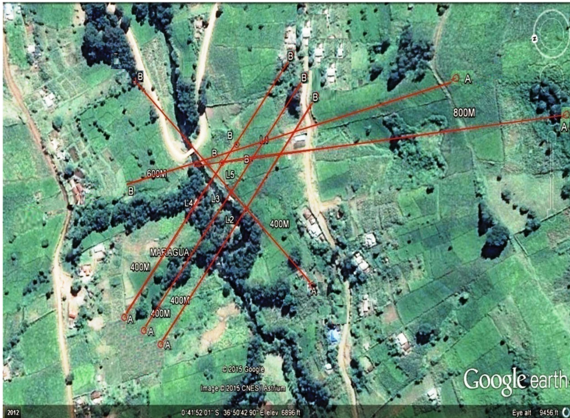
Figure 5.1 Google earth map of Maragua site, showing the six ERT profiles lay out.
