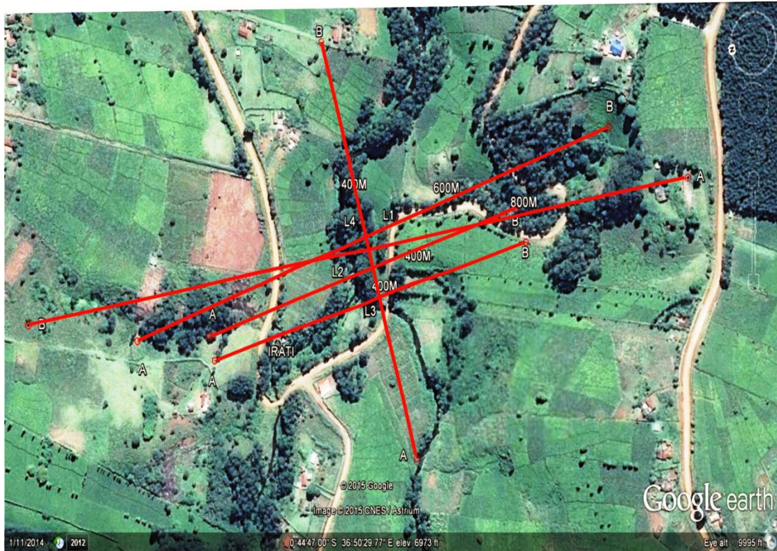
Figure 5.16 Google earth map of Irate site, showing the five ERT profiles layout
