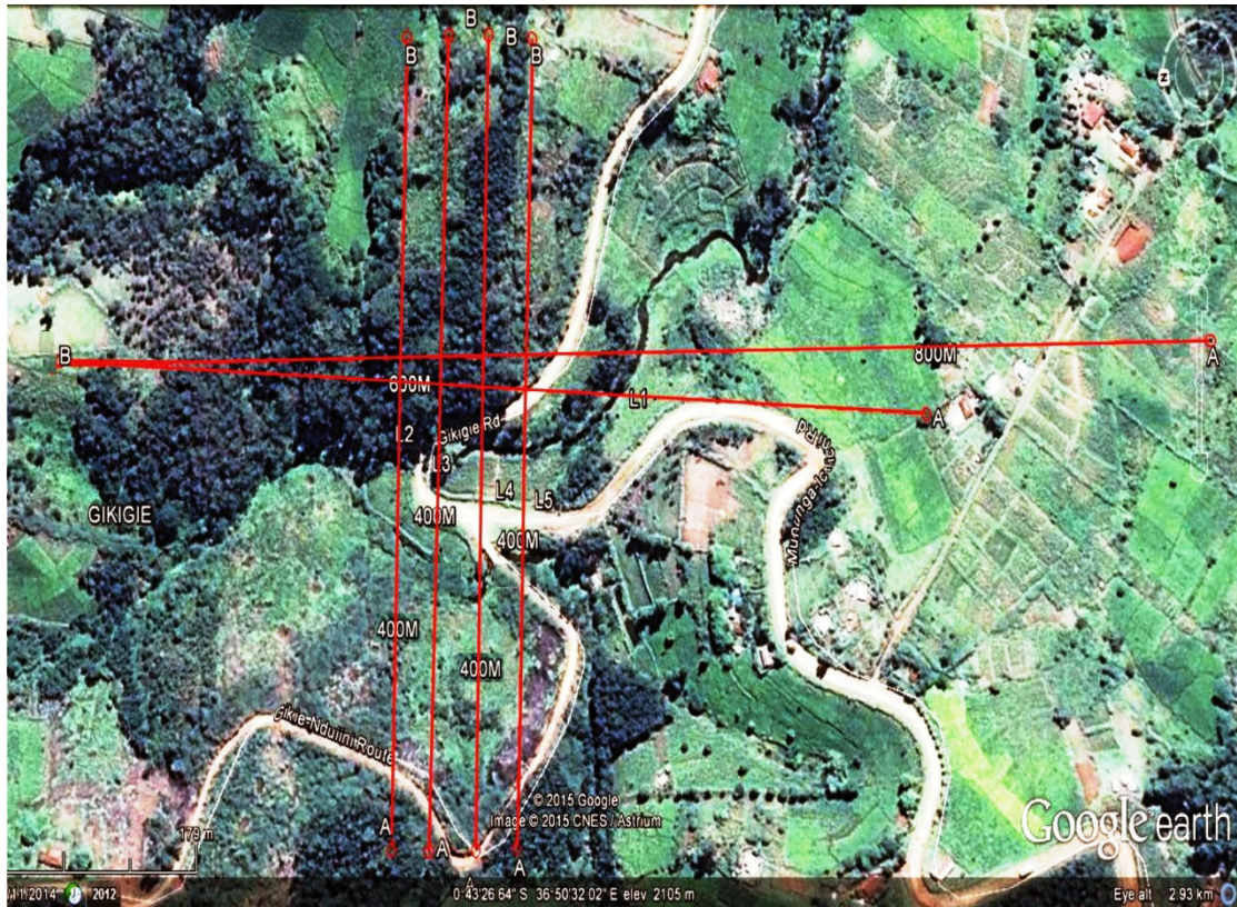
Figure 5.9 Google earth map of Gikigie site, showing the six ERT profile layout.
