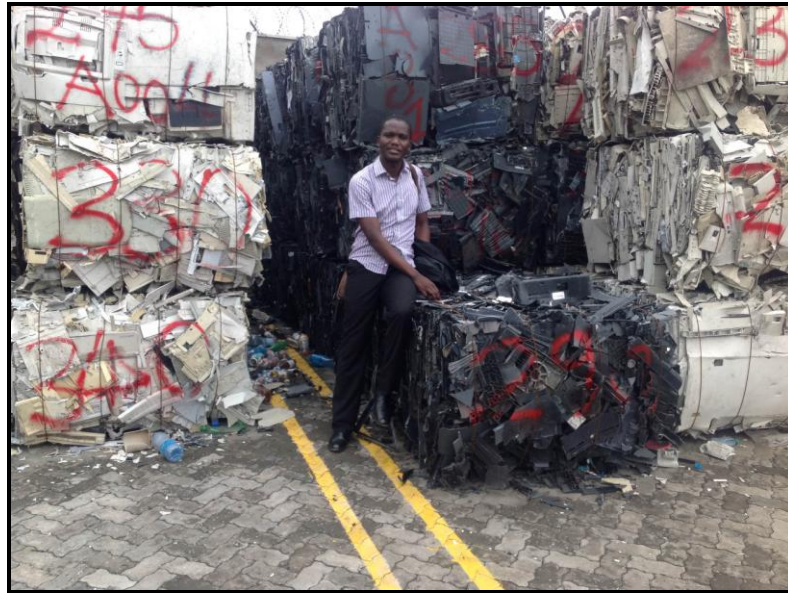
Plate 4-3: WEEE separated, bailed and weighed for exportation by EACR
