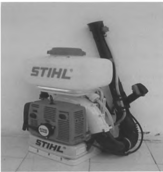
Figure 5. The Stihl 420 motorized backpack mist blower.
