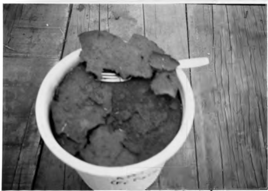
Plate - 2 Surface sealing on Katumani Luvisol
