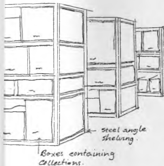
COLLECTION STORAGE UNITS.
