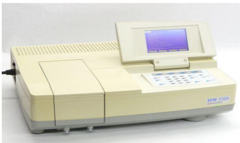
Figure 2.12: UV/Vis spectrophotometer: model UV-Vis UV 1800 Shimadzu
