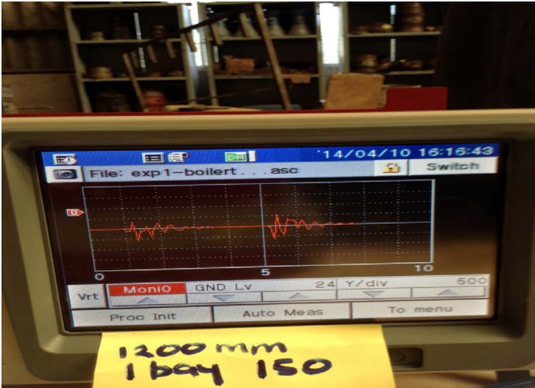
Figure 4.2b-Vibration Results for 1200mm High Unbraced model
