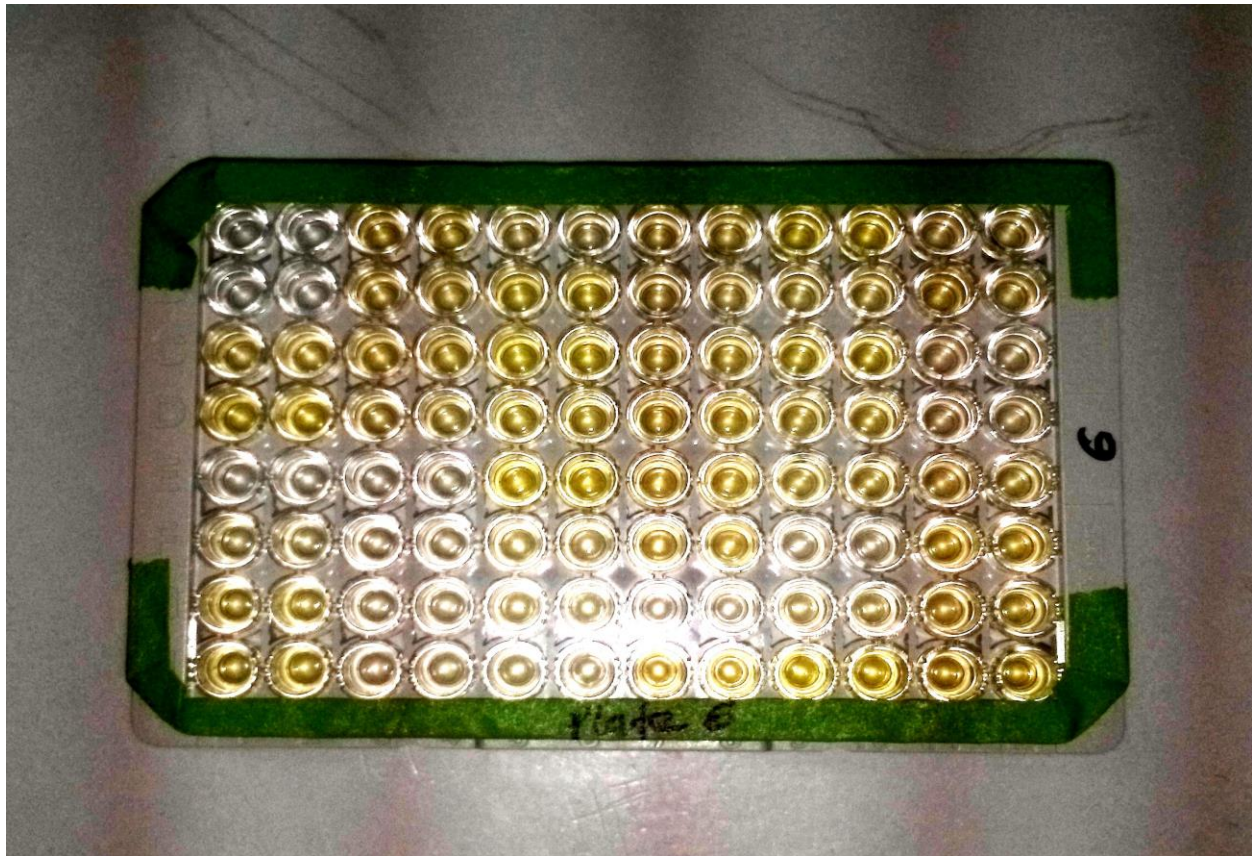
Plate 3.1: A 96-well ELISA plate for screening antibodies to Coxiella burnetii . Note the hue of yellow indicating seropositivity
