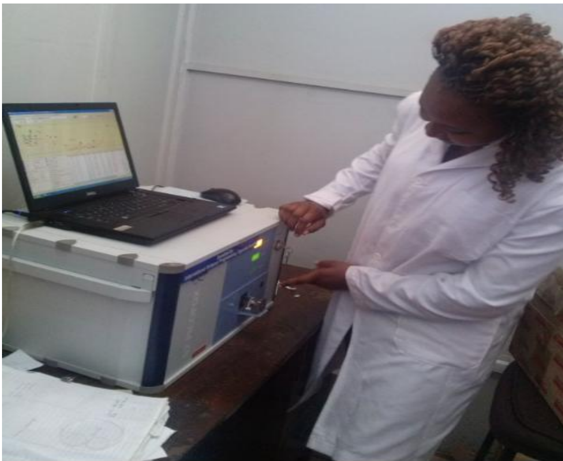
Figure 3.4: Using Total X-Ray Fluorescent (TXRF) instrument to determine heavy metals in the samples.
