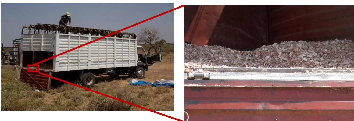
Figure 3.2 Truck floor modified with saw dust
