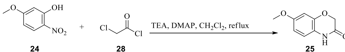
Scheme 2.4: Synthesis of benzoxazines using chloroacetyl chloride
