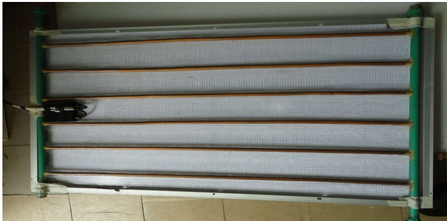
Figure 3.3: Water circulation line behind the PV module
