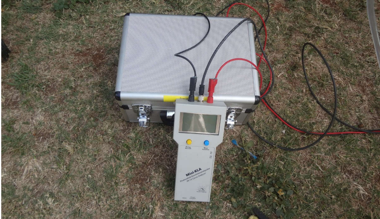
Figure 3.7: Measuring system for taking I-V curve of the PV module (Mini-KLA)
