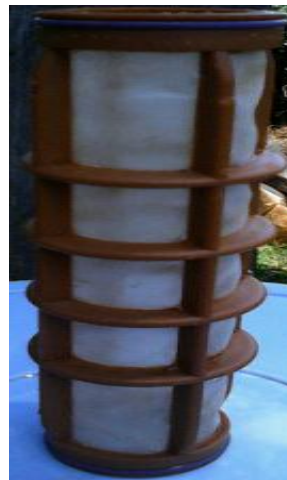
Fig. 4.4(d) Filter after cleaning
