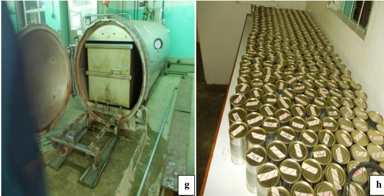
Fig 7. 2: Grain runner bean canning process at Njoro Canning Factory; a) soaking, b) blanching, c) can filling and brining, d) can sealing, e) can cooling after sealing, f) retorting, g) can removal from retort and h) storage
