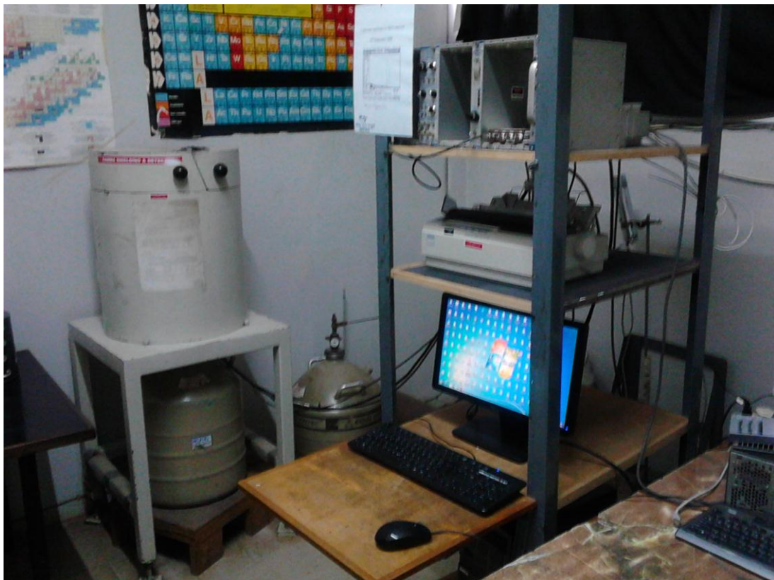
Figure 4-3 Gamma-ray spectroscopy unit at the Institute of Nuclear Science and Technology, University of Nairobi
