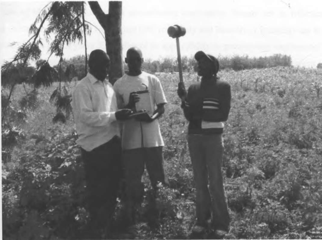
Fig 4.9: The author taking magnetic data in the field using MP2 SCINTREX proton precession magnetometer
