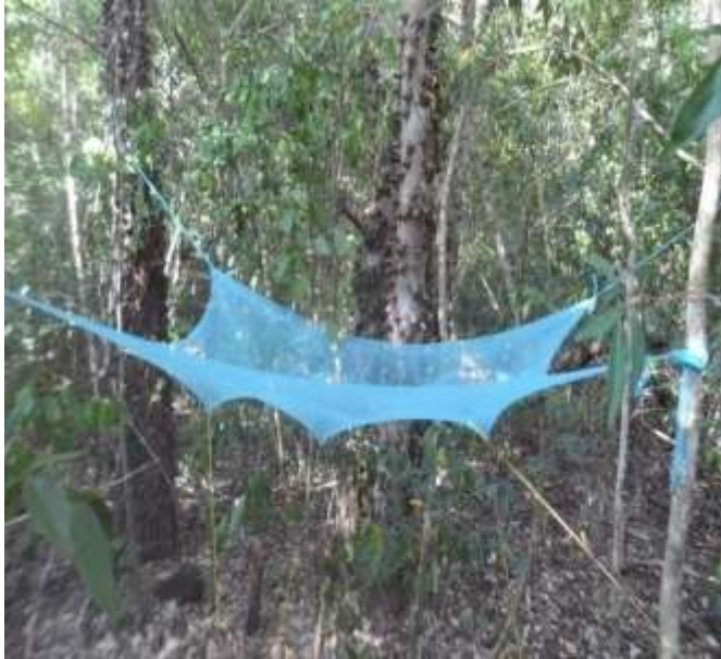
Plate 2: Seed trap design used in the study for seed rain estimation
