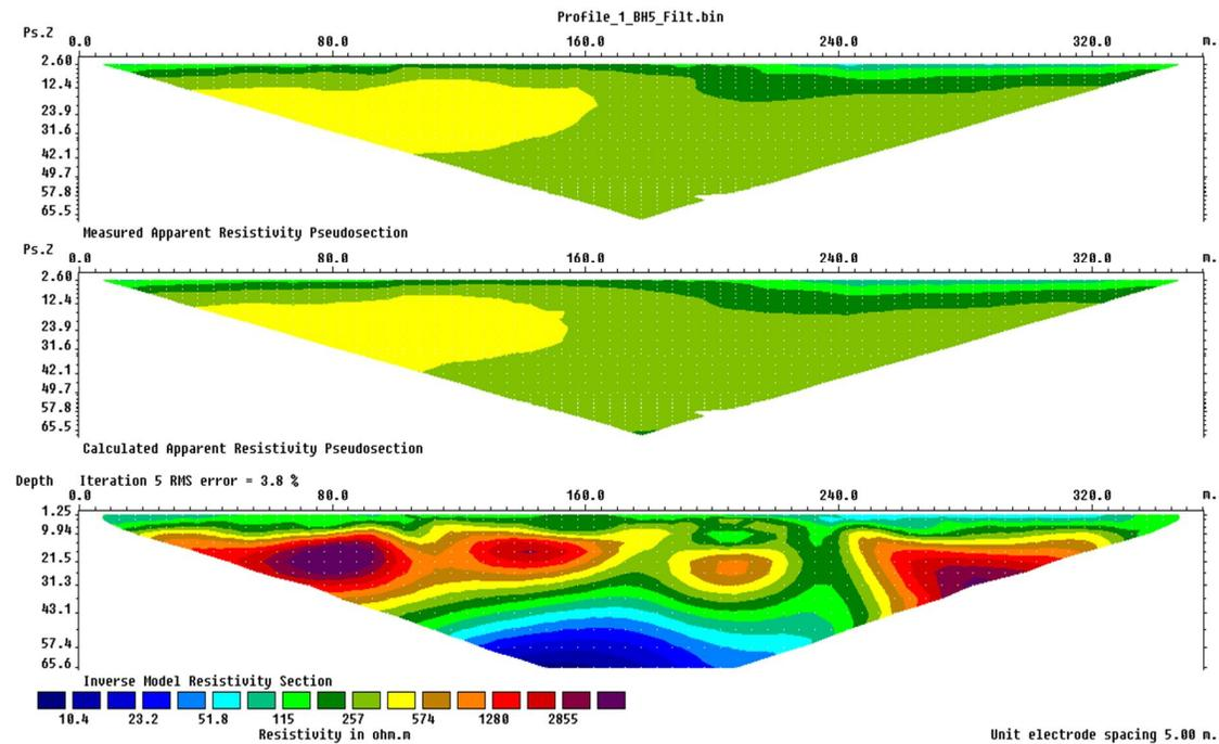
Figure 3. 6: Profile 1 showing the vertical slice obtained from borehole 5. (After Barongo, 2008).
