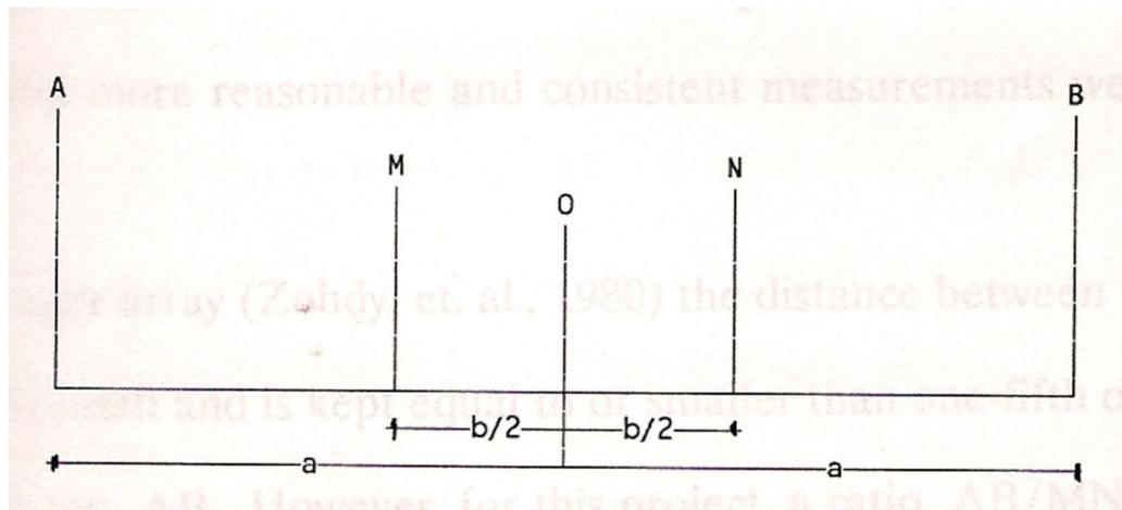
Figure 2. 1: Schlumberger electrode configuration, (After Das, 1995).
