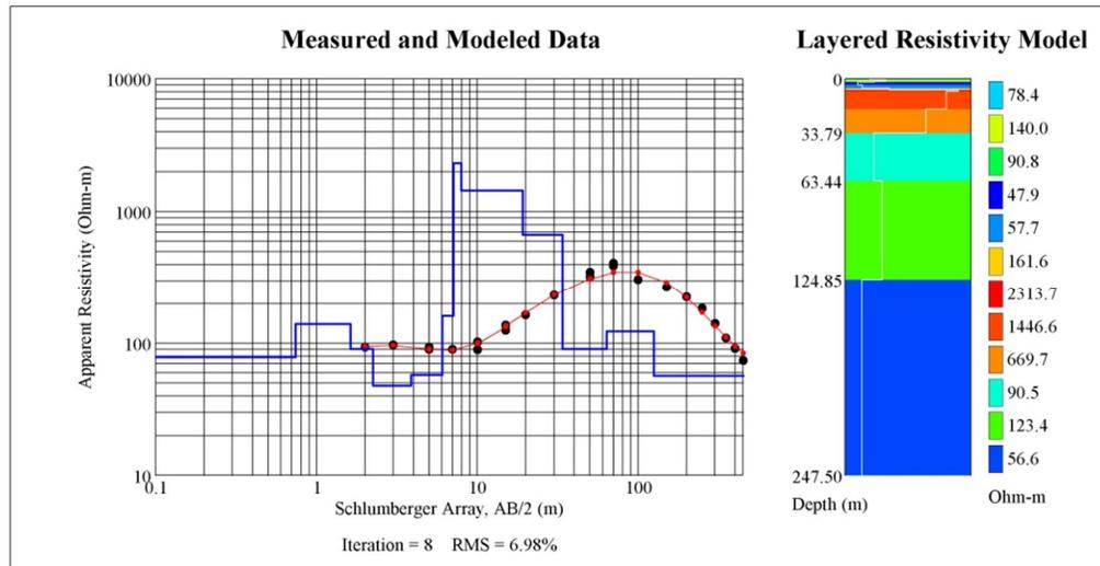
Figure 3. 2: Interpreted sounding results for borehole 2. (After Barongo, 2008).
