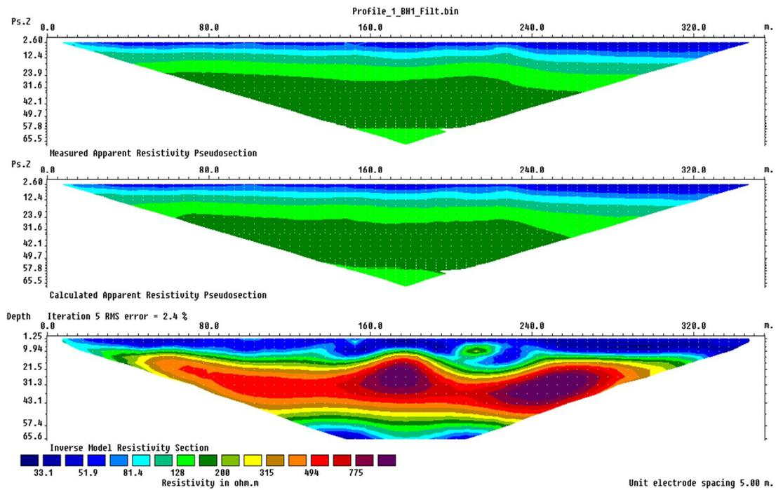
Figure 3. 5: Profile 1 showing the vertical slice obtained from borehole 1. (After Barongo, 2008).
