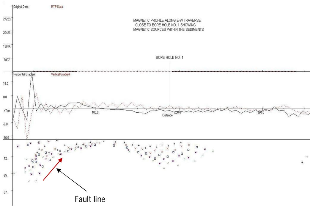
Figure 3. 7: Magnetic profile result along borehole 1.(After Barongo, 2008)
