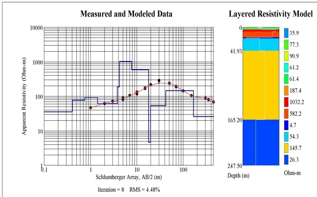
Figure 3. 1: Interpreted sounding results at borehole 6. (After Barongo, 2008).
